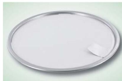
The ring with a whole easy peel lid is manufactured from alufoil, supplied by Amcor Flexibles. The lid is heat sealed to the inner parts of the Easy Peel® ring and both the PP layers of the alufoil laminate and the ring melt and merge while cooling to give a 100% barrier against oxygen and light. Both the PP layers of the alufoil laminate and the ring melt and merge while cooling to give a 100% barrier against oxygen and light.
