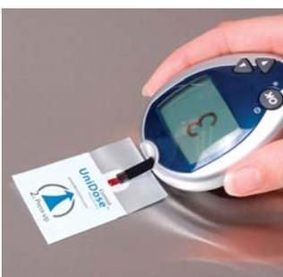
Current PE vials used for glucose control solutions achieve 18-24 month stability for an unopened vial, but only three month stability once the vial has been opened. The single format alufoil-based UniDose, with its very low water vapour transmission rate, allows a very small volume of control solution to maintain glucose concentrations within specification for 24 months at up to 30 °C.
