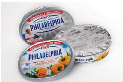
A special punching process was developed by Constantia Teich featuring eye mark steering to punch lids in register to the partial embossing. The eye mark is applied by the embossing roller which avoids the use of a printing machine and saves cost for the customer. The un-embossed sealing rim provides optimum sealing and peeling characteristics.
